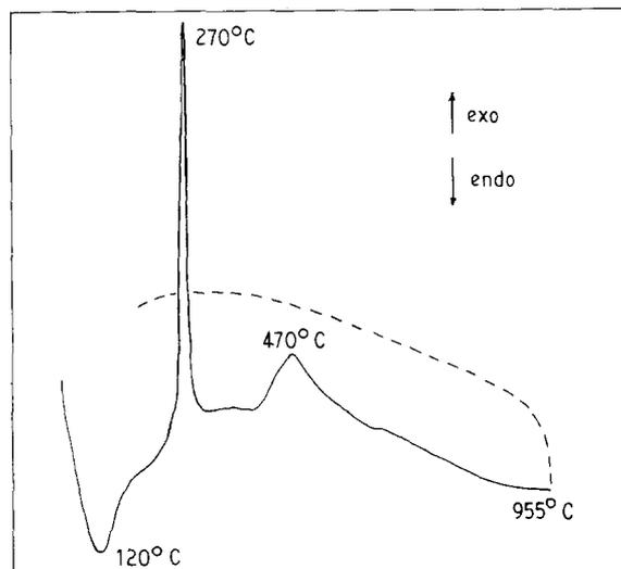
Figure 1 Typical DTA curve for a gel dried at 110 °C (sample 1).
