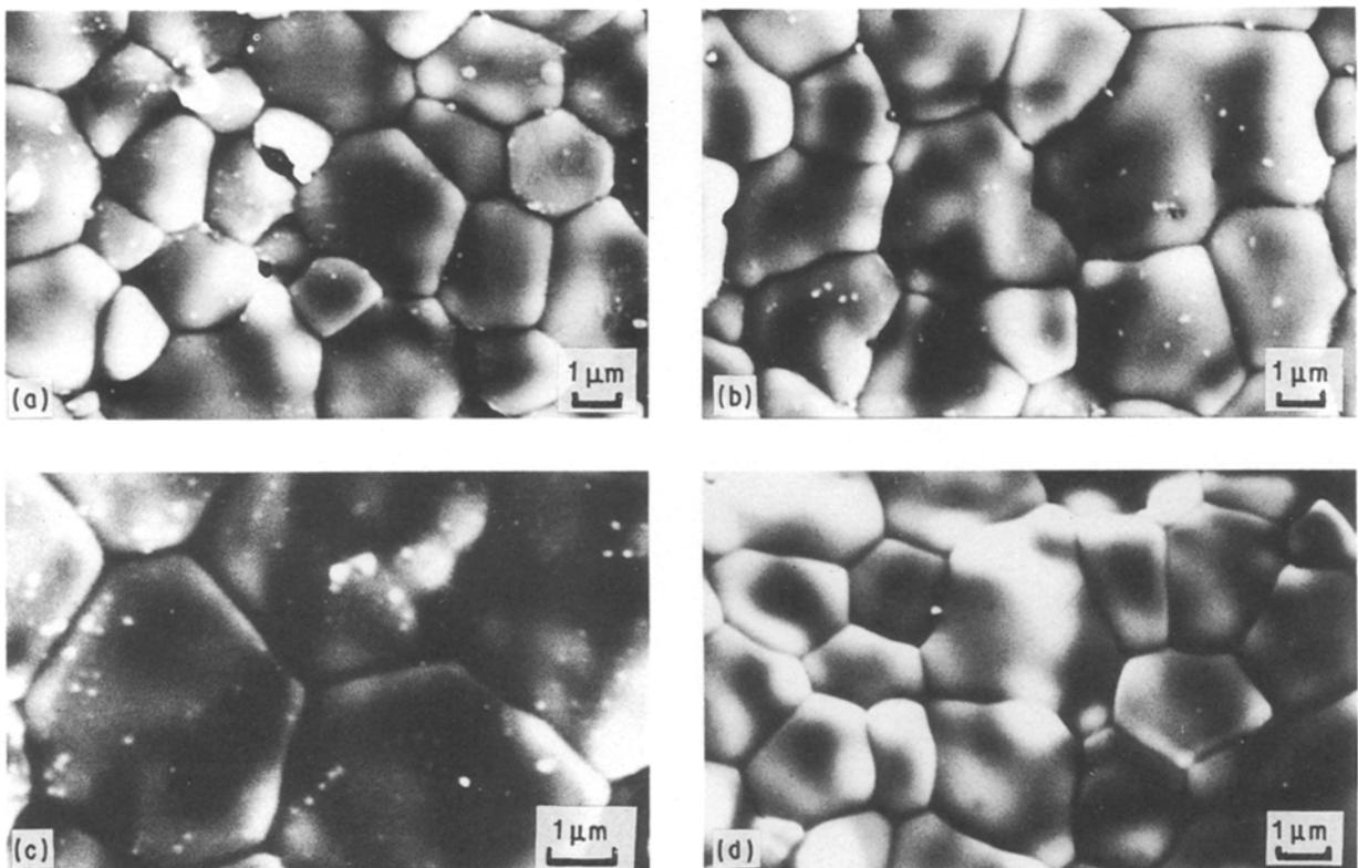
Figure 6 Scanning electron micrographs of the natural surface of sintered YSZ samples. Samples: (a) 3, (b) 5, (c) 6, (d) 7.
