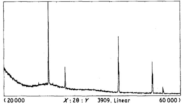
Figure 5 X-ray diffraction pattern of a ceramics sintered at 1420 °C (sample 4).
