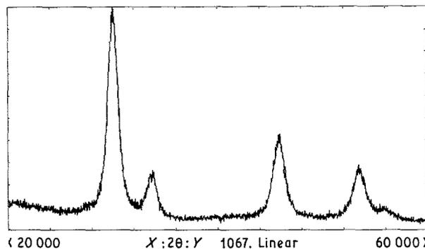
Figure 2 X-ray diffraction pattern of sample 4 after 500 °C calcination.
