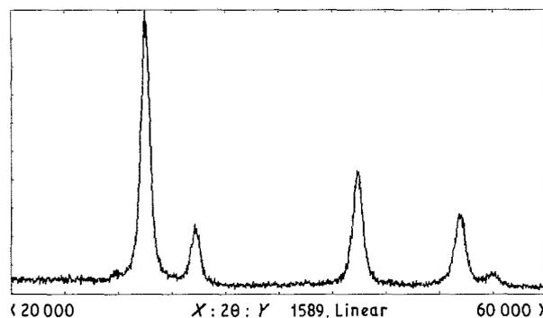
Figure 3 X-ray diffraction pattern of sample 4 after 700 °C calcination.
