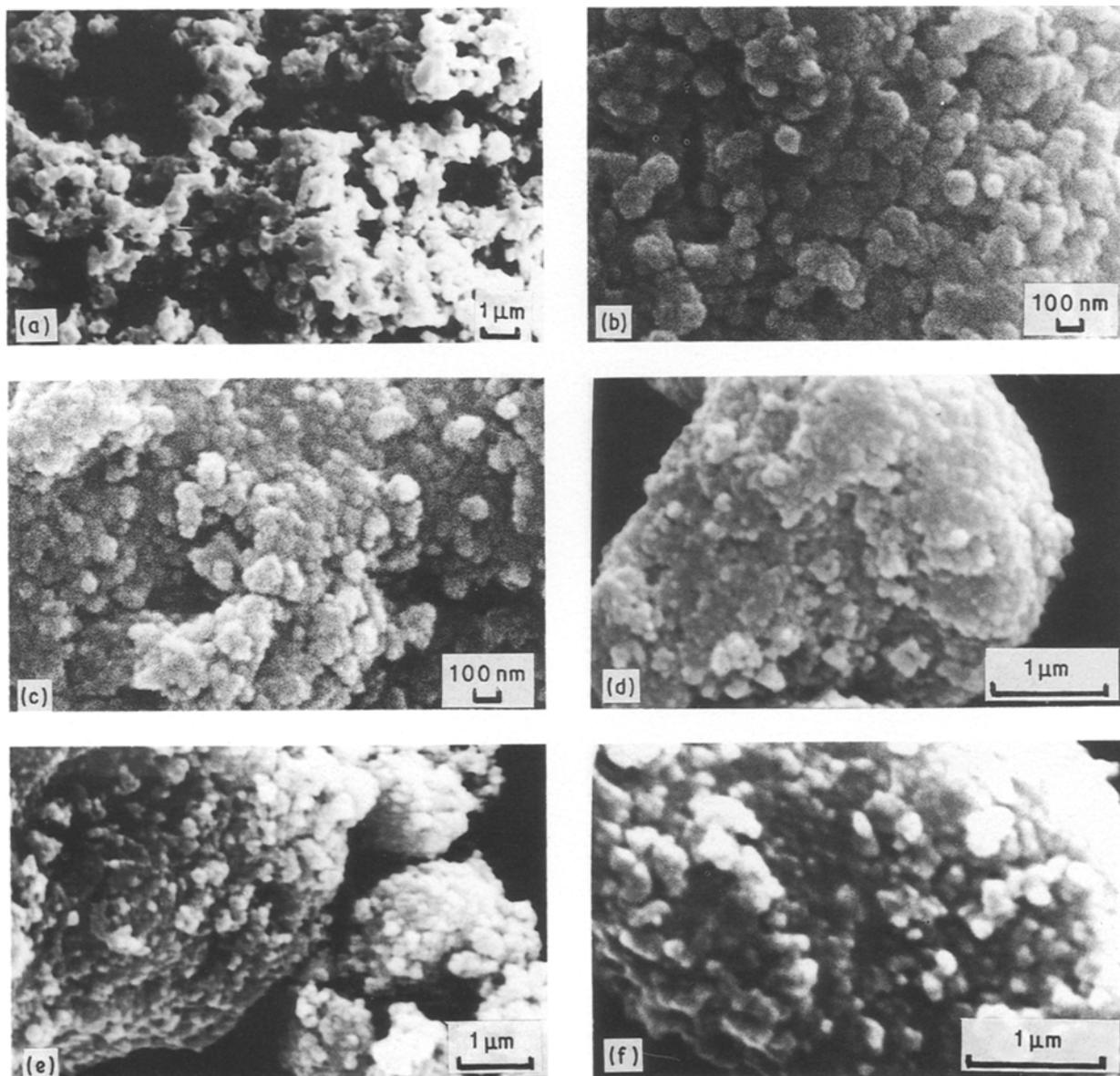
Figure 4 Scanning electron micrographs of powders calcined at 700 °C for 4 h. Samples: (a) 1, (b) 3, (c) 4, (d) 5, (e) 6, (f) 7.
